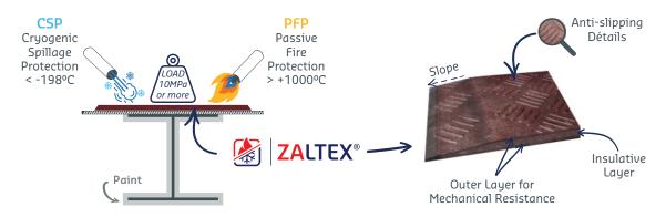
Design example for two hours CSP resistance with low thickness (21mm) and density (18 kg/m³)
